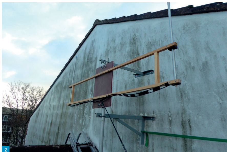
Fig. 1: General arrangement of end-fire array. Fig. 2: The support structure of the end-fire array antenna shown with the telescopic rods retracted. Fig. 3: 4m version with croc-clips in place temporarily. Fig. 4: Balanced ATU circuit.
