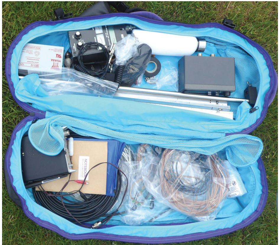
FIGURE 6: The skateboard bag I used for a day trip, with everything I needed including water, transceiver, 20-10m ground-plane antenna (a), and the antenna deployed out in a field north of Brighton (b).
