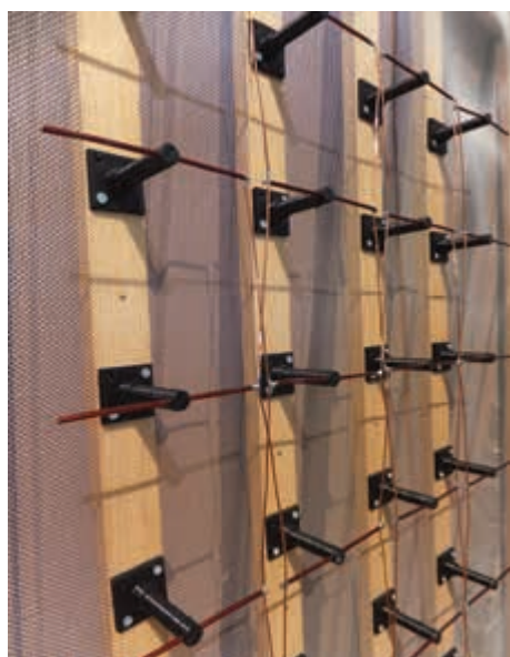
PHOTO 8: 23cm collinear array of dipoles mounted above a reflecting metal mesh using \frac{1}{4}\lambda -high 3D printed supports.
