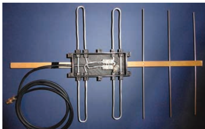
PHOTO 12: A 3D printed case (here with lid off) protects the matching components and firmly holds the driven elements of this ZL Special.
