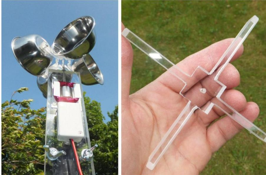
**4 cup wind generator** – shown above is a simple 4-cup wind-generator (anemometer) I made from Perspex using a router, band saw, set of drills, files and other tools. The cross piece that holds the cups is tricky for a beginner to make by hand. It's not easy with hand tools to make sure the shaft channel is straight and true, so I decided make a 3D printed version to compare.
